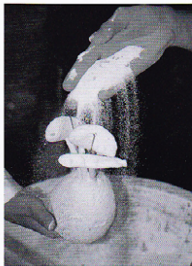
11. First Layer. Application of the grade of alumina
