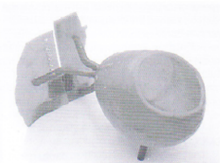
9. Microfusion by attached crucible. The Pouring Tree
