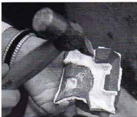
14. Cleaning the mold
